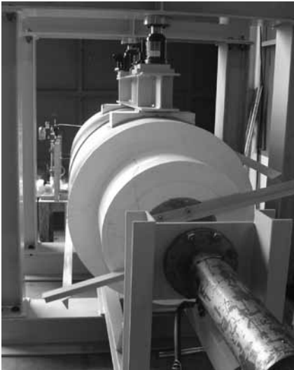
Full scale test of 24" NB (600NB) cryogenic pipe shoe at -165°C for client approval.
